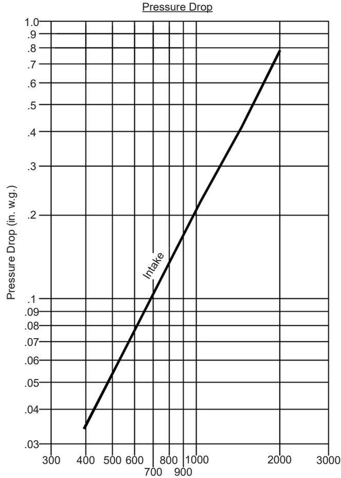
Intake air converted to standard air density.
